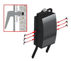
5) Push adapters from the reverse side of the loudspeaker "Banana". Then, place two rubber rings on each side of the loudspeaker between the adapters and the fastening thread.
