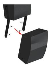
6) Insert two of the adjustable clamping levers (type GN 300-63-M10-25-SW) from the outside through each of the adapters and the rubber rings and finally screw them into the corresponding mounting threads of the loudspeaker.
