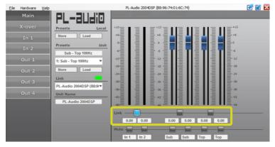
For the respective outputs, the mixer selects which input signal is used at which level. When using the output for a subwoofer, we recommend using the input signal from both inputs. For stereo localization, the input channel that is signal-relevant for the respective output is used (e.g. input A for left  $\rightarrow$  in the mixer input A to the desired value, while input B is set to "mute" using the fader).
