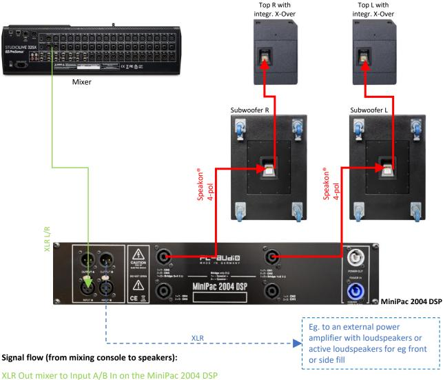
Thru A/B from MiniPac 2004 DSP to external amIplifier or active speakers Speakon® CH 3/CH 4 to Subwoofer R (2+/2-) Speakon® CH 1/CH 2 to Subwoofer L (2+/2-) Speakon® from Subwoofer R to Top R (1+/1-) Speakon® from Subwoofer L to Top L (1+/1-)
