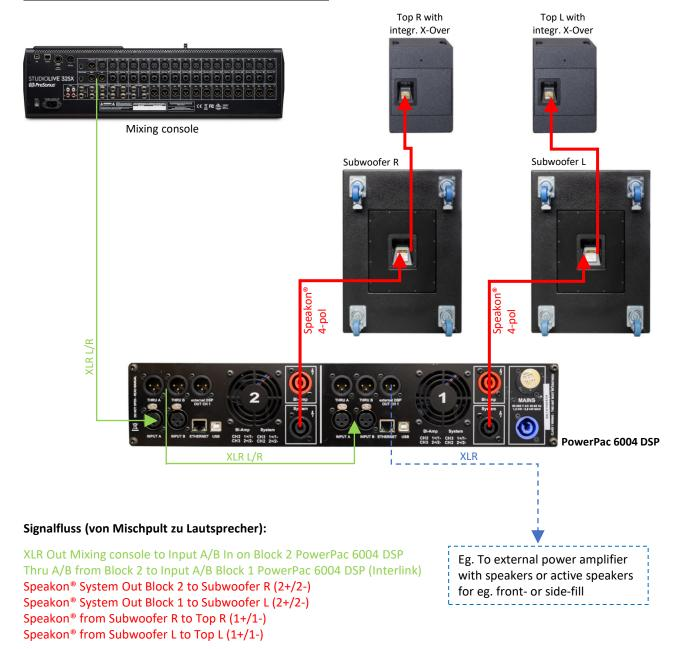
In the above example, the PowerPac 6004 DSP supplies up to 2 basses at 8 ohms (2500 W) and up to two tops with integrated crossovers at 8 ohms (800 W) per power amp block. For the sake of simplicity, only one subwoofer and one top per side are shown in the example graphic.
