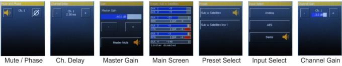
When the user navigates to a screen other than the Main Screen by swiping, the display returns to the Main Screen after 25s.
