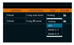
The same procedure can be used to change the active audio input. The following pictures shows all available audio input types. Depending on the device, there may be less audio inputs available.
