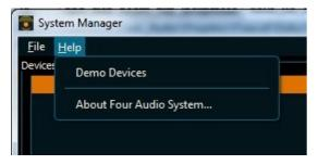
Simply check the "Demo Devices" menu entry. The devices list will be populated with a number of devices with connection type "virtual".
