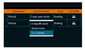
In the System Manager window, double click on the "Current Preset" column for the desired device. This activates the drop-down control inside the table.
